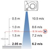
According to standard NSF-37-2012, the maximum installation height is the speed profile point at 8,14m/s plus 0,9m. So FLY K can be used until 1,15m+0,9m=2,05m.
